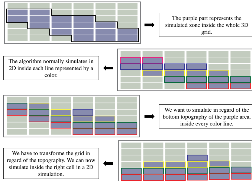
Figure 8 – Vertical cross-section of a 3D grid that is transformed regarding the bottom altitude of its simulated zone.
