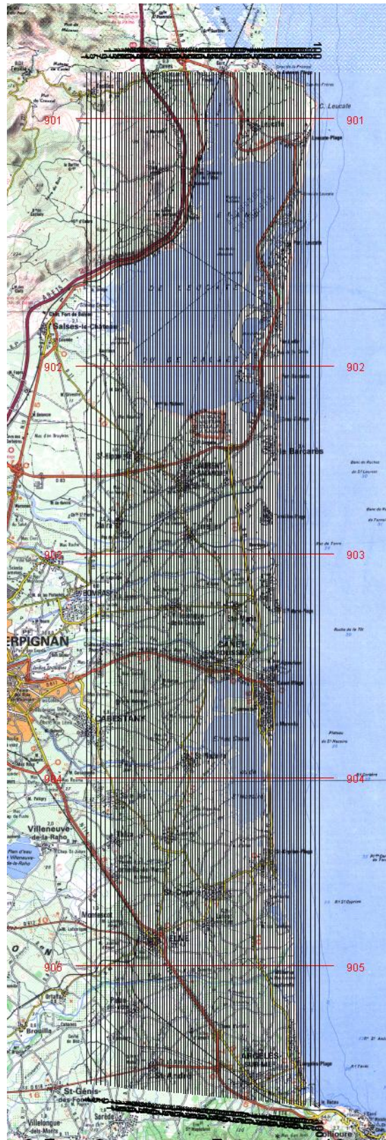
Figure 1. Flight line plan plotted over topographic map. The start (original) survey plan comprises 91 flight lines at 100 m spacing, except in the west and east. The final plan used 100 lines at a spacing of 100 m,
