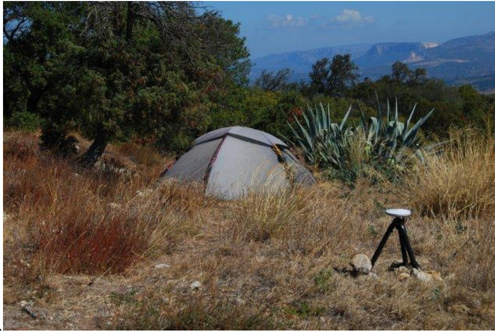
Figure 12. The base station tent and GPS receiver at their location in village of Chateau de Caladroy. The magnetic sensor was located among the bushes for protection against strong winds. Photo: Rob Cuss
